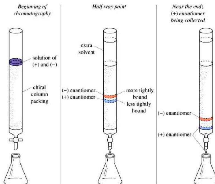
**Figure 4:** Schematic diagram of chromatographic separation of racemic mixture
