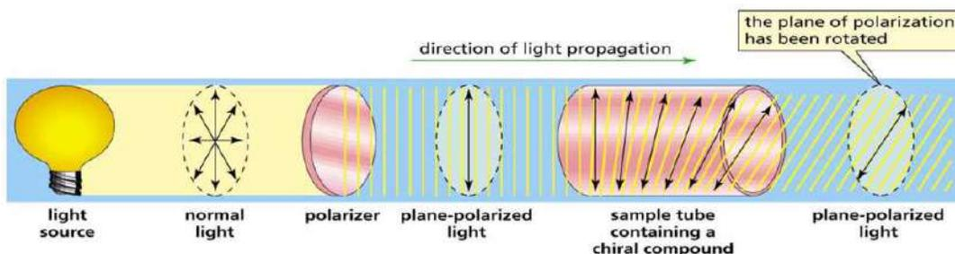
**Figure 1.** Schematic representation of simple polarimeter
