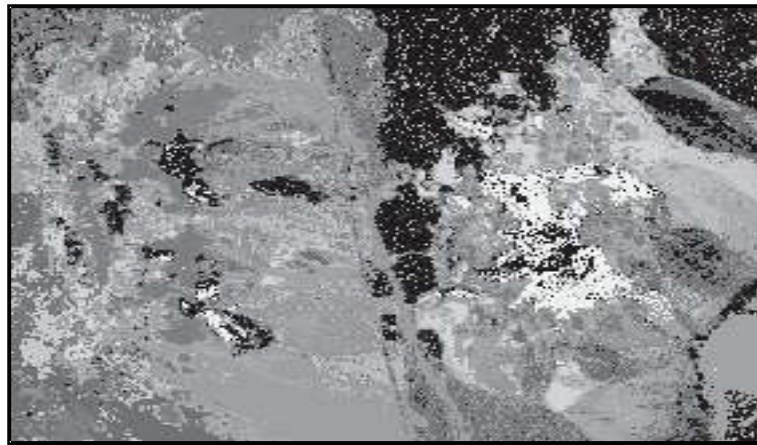
Figure 2.23 Classified Image of 1995 AVIRIS Frame Over Cuprite, Nevada Using Spectral Unmixing Techniques
