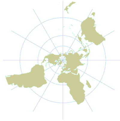
Fig. 3.22: Polar azimuthal stereographic projection is a planar projection with a conformal property.
